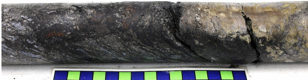
Figure 3: Core photo from RK-25-280c1 displays semi-massive, off-scale (>61,000 cps) from uranium vein at 834m down hole
