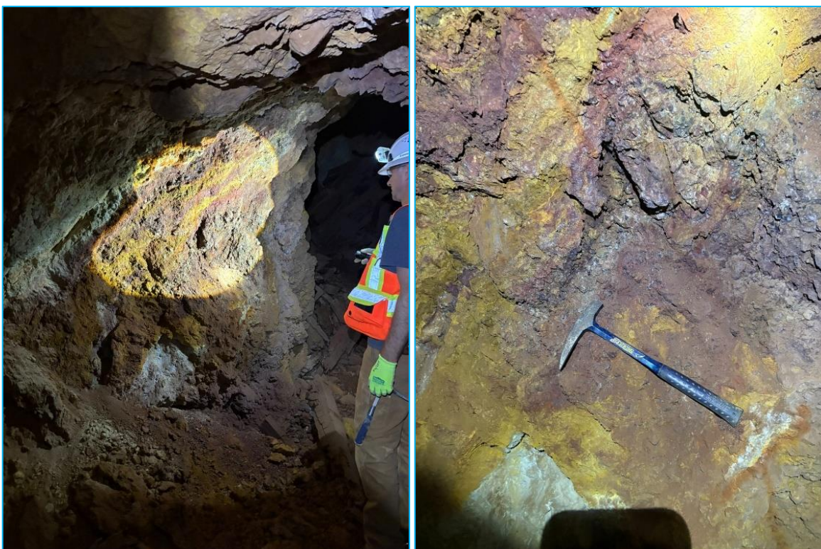
Figure 1: Extensive limonite after sulphide in fault breccia zone with quartz veins 2 .
