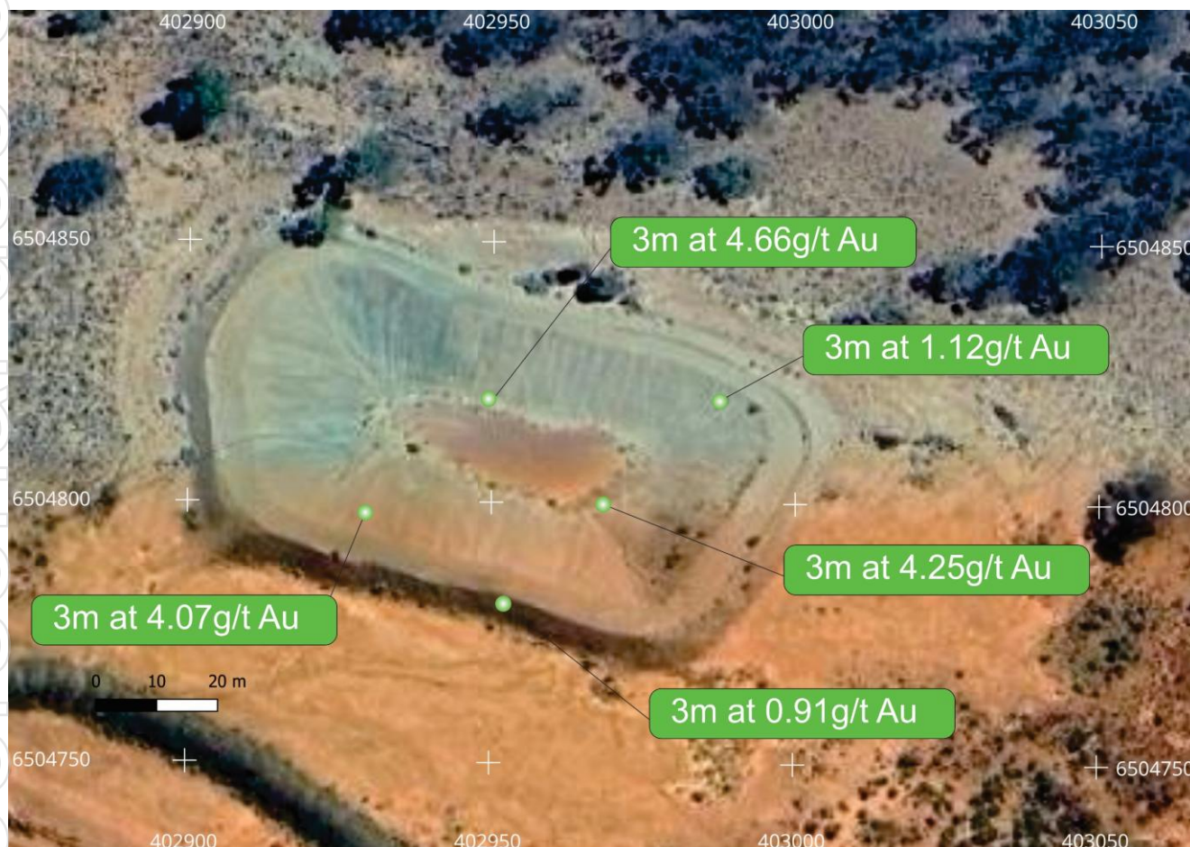
Figure 5: North East Tailings Dam Drilling Results (Pre-Relocation)
