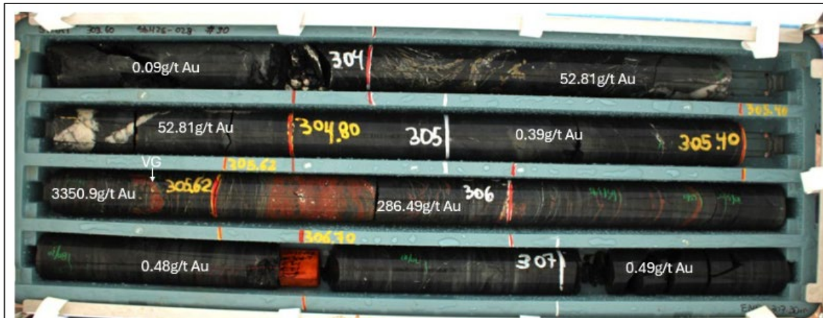
Plate 1 - SDH25-028, 305.4 - 306, Hematite-Magnetite alteration and high Au grade
