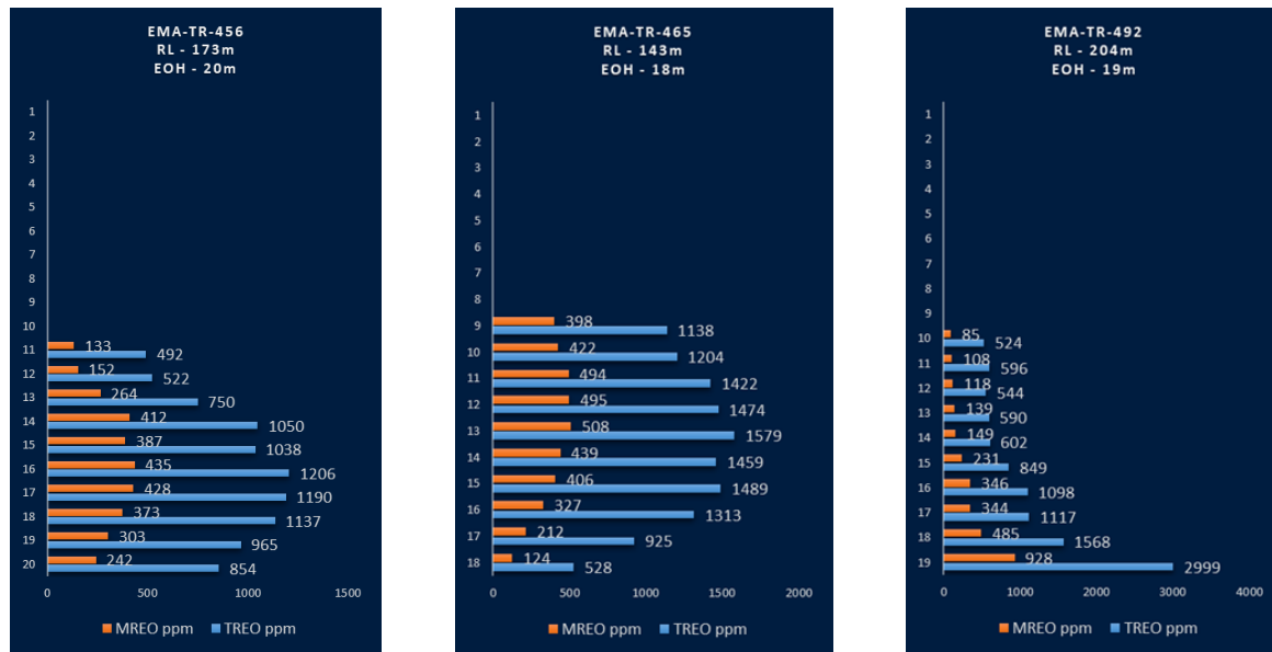
Figure 4 – Drill-hole profiles showing typical ionic REE enrichment zone with high NdPr grades close to the fresh rock interface.
