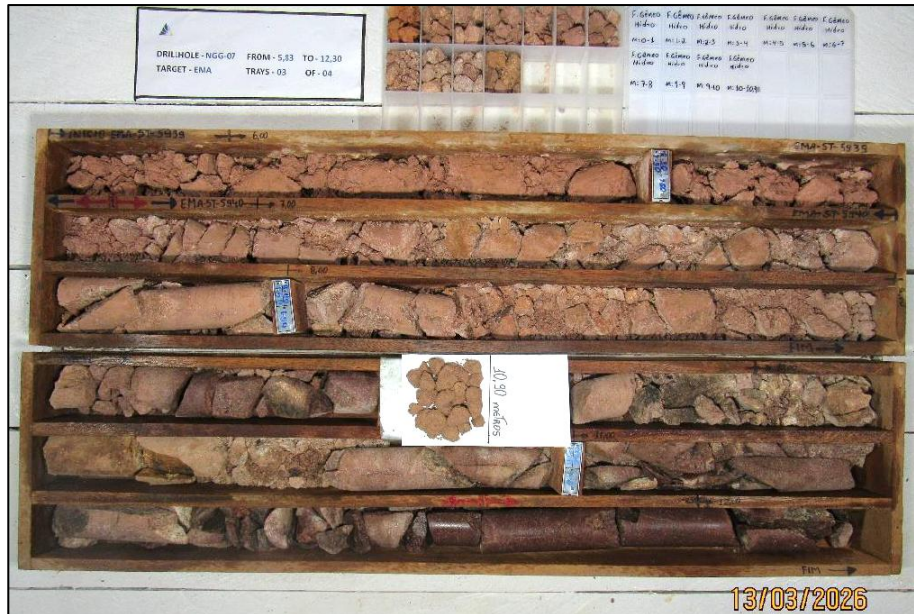
Figure 5 – Drill core from hole NGG-07 drilling to a final depth of 26m, intercepting solid felsic volcanic bedrock at 11.75m. This hole was drilled for physical core only. No assaying of samples has been completed and no interpretation of grade can be inferred from the physical core.
