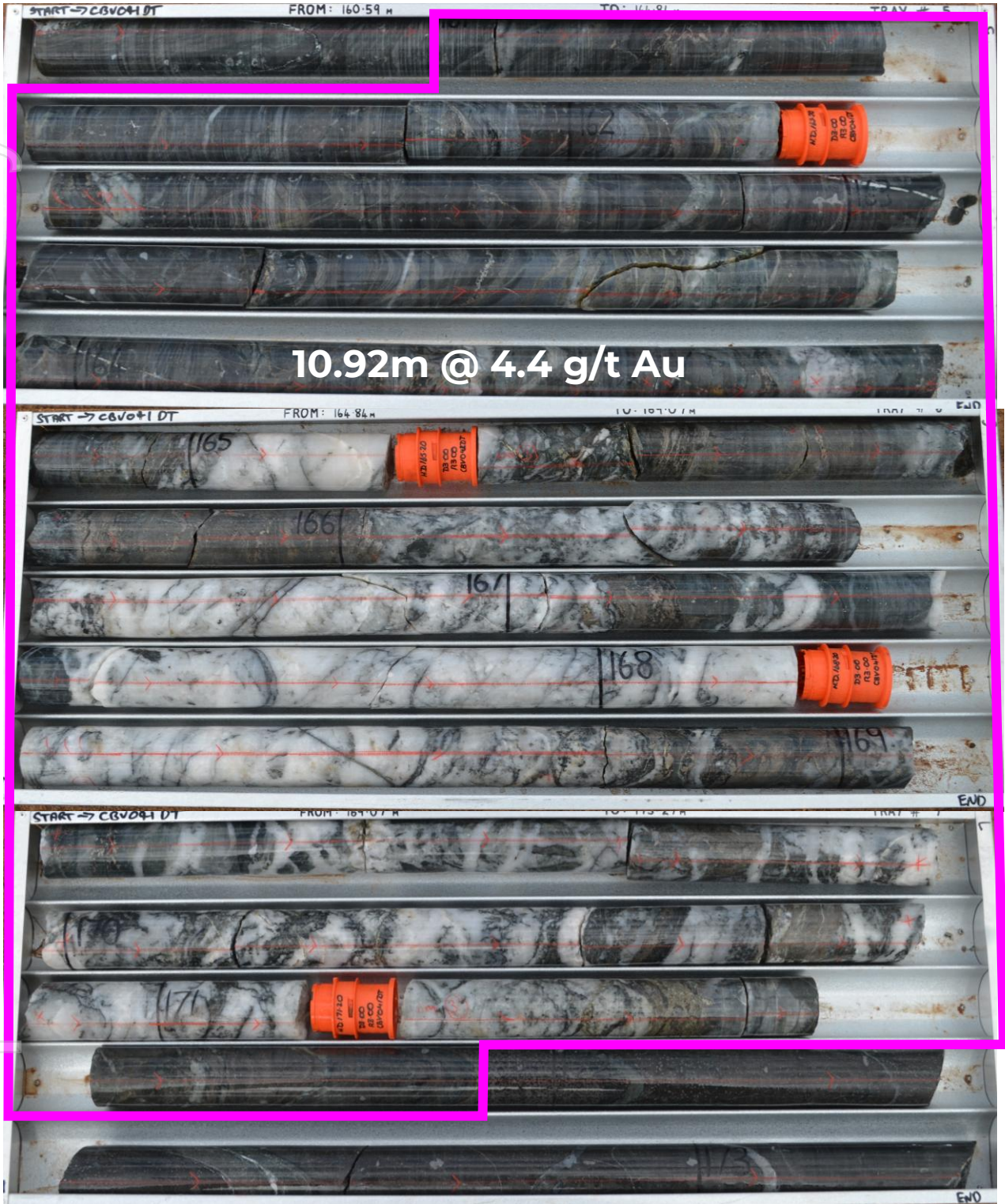
Figure 3: Typical vein-style high-grade gold mineralisation at Blue Vein, 10.92m @ 4.4 g/t Au from 161m (CBV041DT)
