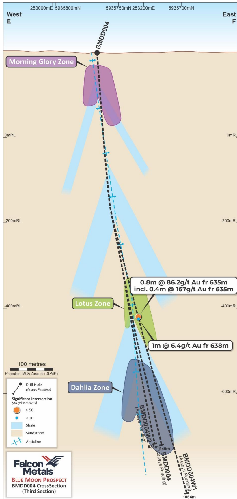
Figure 7 BMDD004 (Third Section) - schematic cross section looking north showing the intercept in the Lotus Zone
