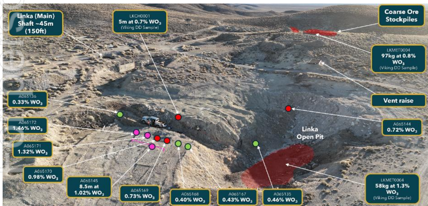
Photo 1: Linka (Main) Pit and location of historic samples. Note the Linka Pit has been partially backfilled, so sample locations are approximate and under cover.
