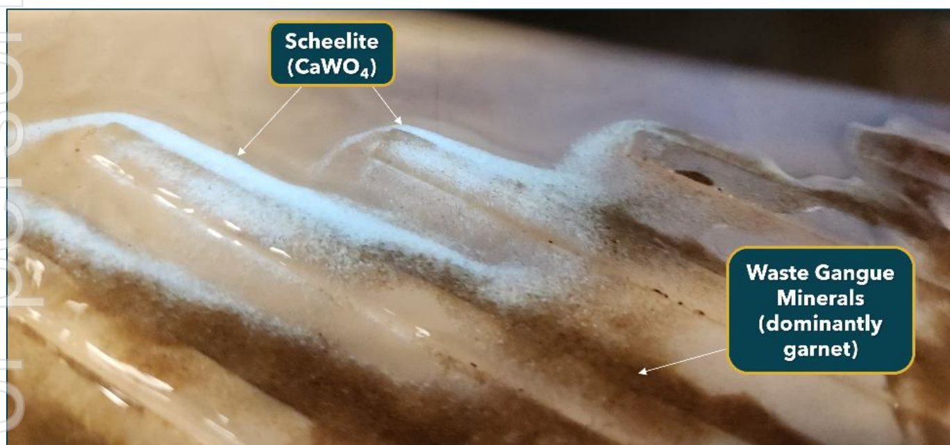
Photo 2: Showing separation of scheelite from waste minerals during Wilfley table gravity concentration stage. Assayed grade of Wilfley table product ~18% WO_3 , which feeds into the Mozley table cleaning stage.
