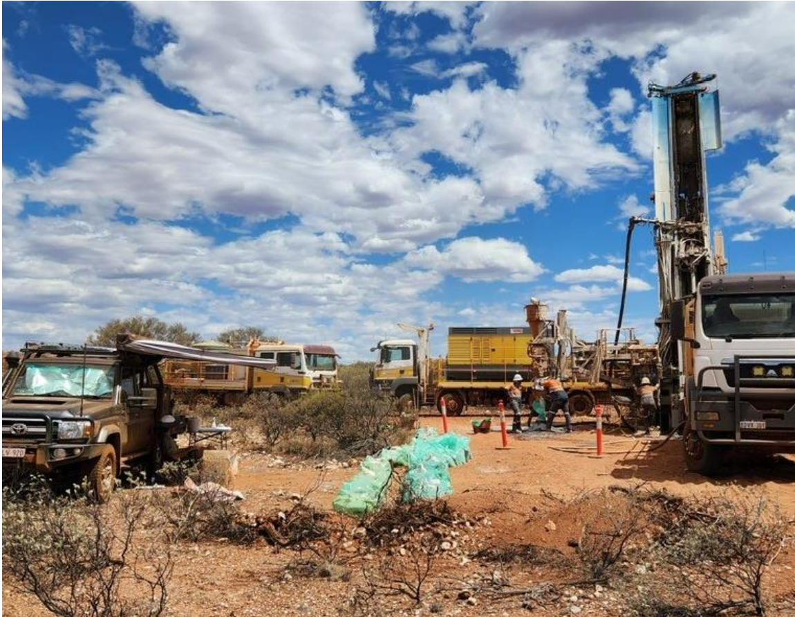
Figure 4: Ausdrill RC rig set up on a Degruassa West drillhole testing soil anomalism.
