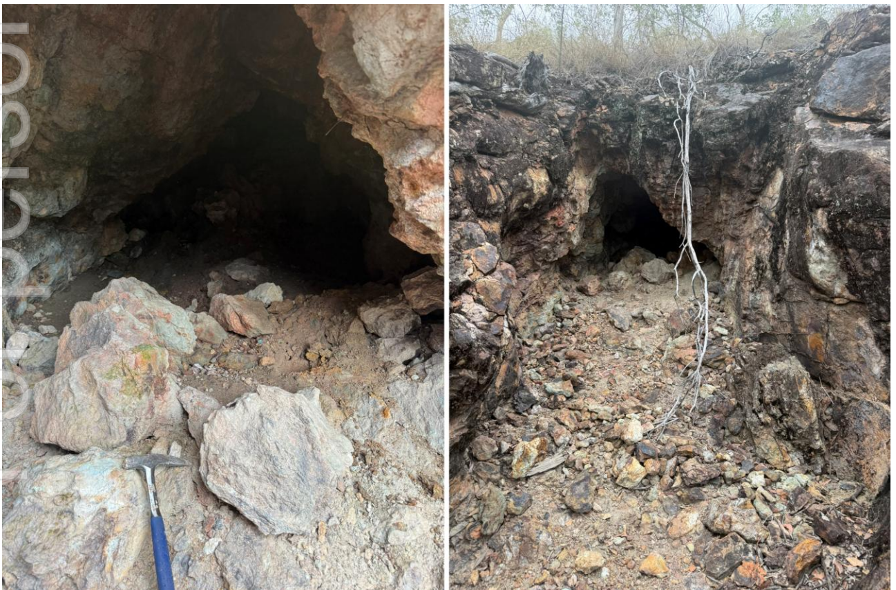
Figure 12 Left: Close up of a mine adit showing malachite on rocks that had fallen from the roof. Right: A mine entry adit on a 1.5m wide vein (same mine adit as the close up photo - Left).
