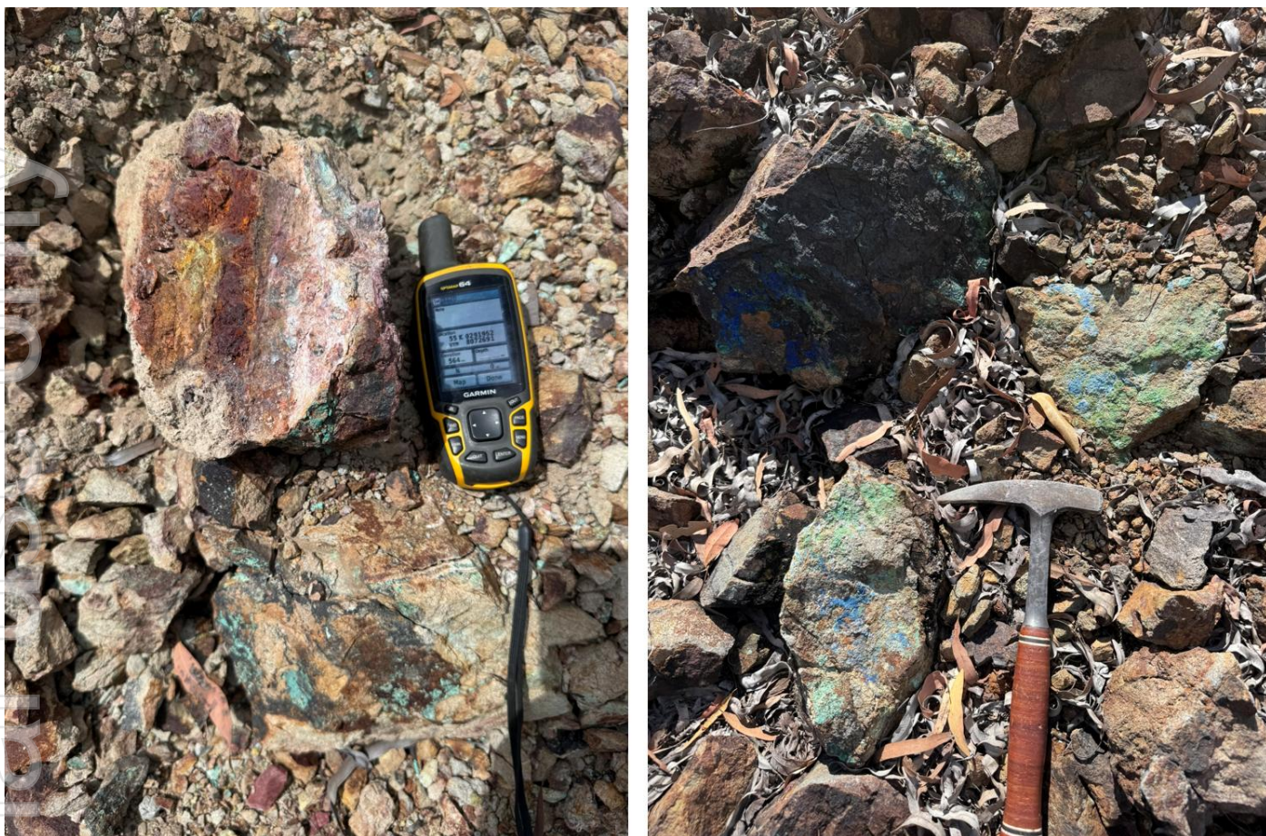
Figure 7 Left: gossanous vein material from the main line of workings – XRF: 1.4% Cu, 142 g/t Ag, 52 g/t In. Right: malachite and azurite on the mine dumps, far eastern vein at Copper Hills.
