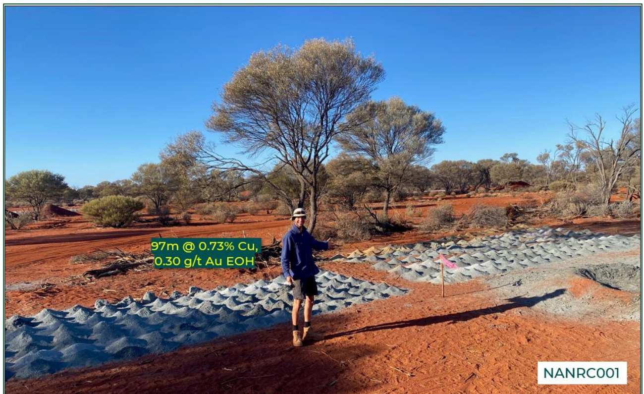
Photo 5. Typical RC drill samples (NANRC001) 1 at Nanadie. Note limited oxidation profile below shallow sandy soils.
