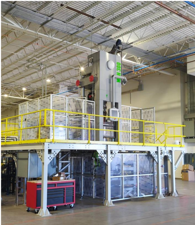
Figure 8: Six-axis 300-ton SACMI press and cold isostatic press
