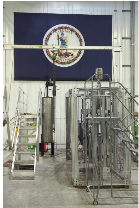
Figure 8: Six-axis 300-ton SACMI press and cold isostatic press
