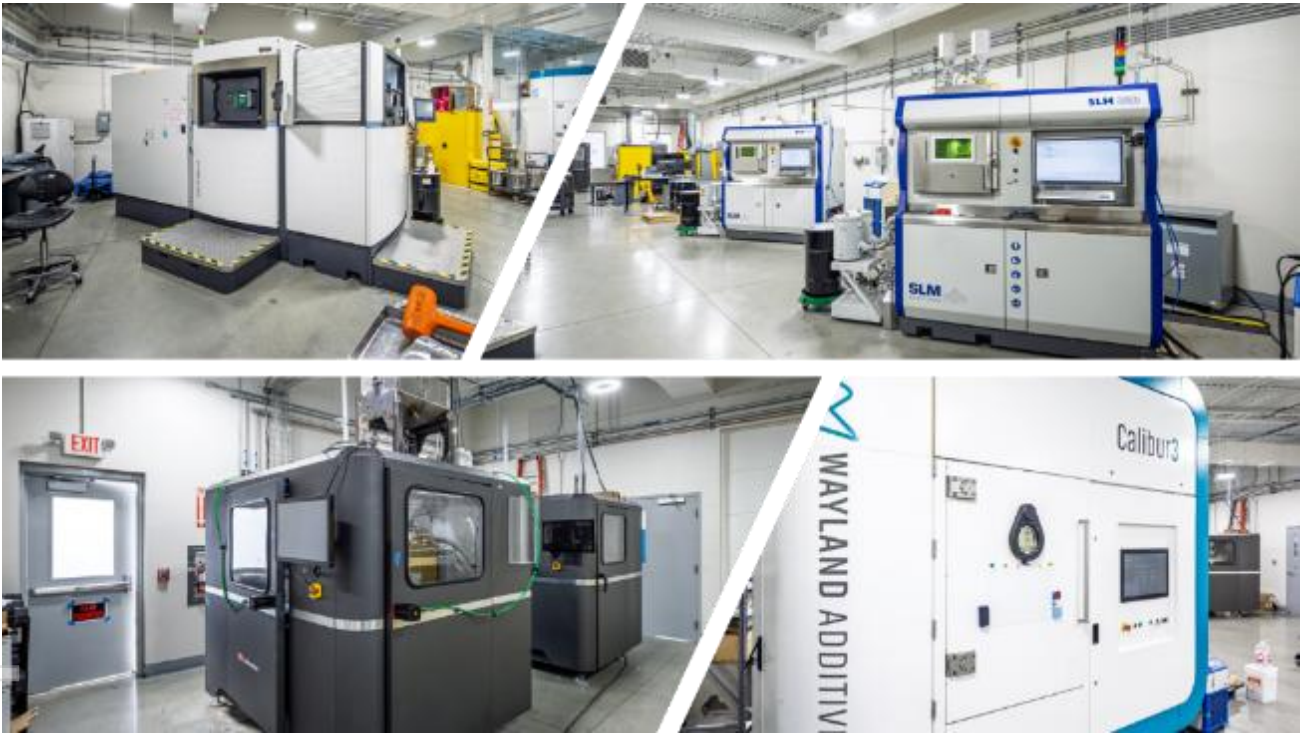
Figure 9, clockwise from top left: 1x EOS LPBF machine, 2x SLM LPBF machines, 1x Wayland Additive eBeam machine, 2x Desktop Metal binder jet machines
