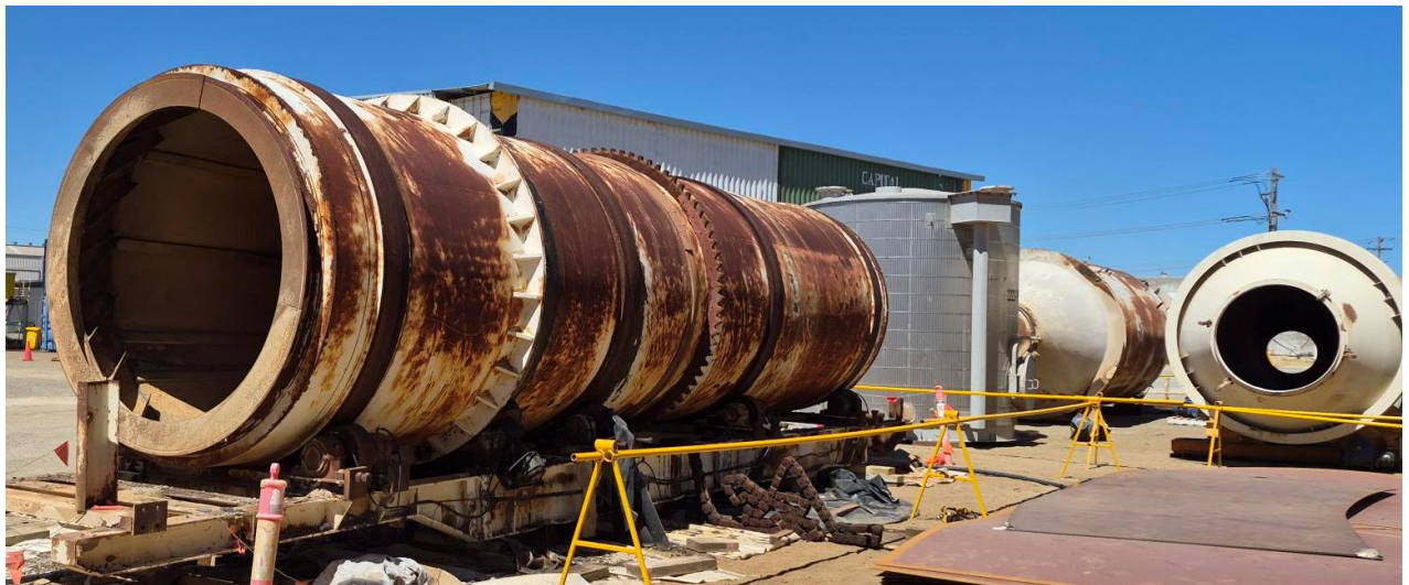
Figure 5: OzAurum agglomerator drum, cyanide tank, lime + cement silos at Polaris Engineering Services Henderson Facility
