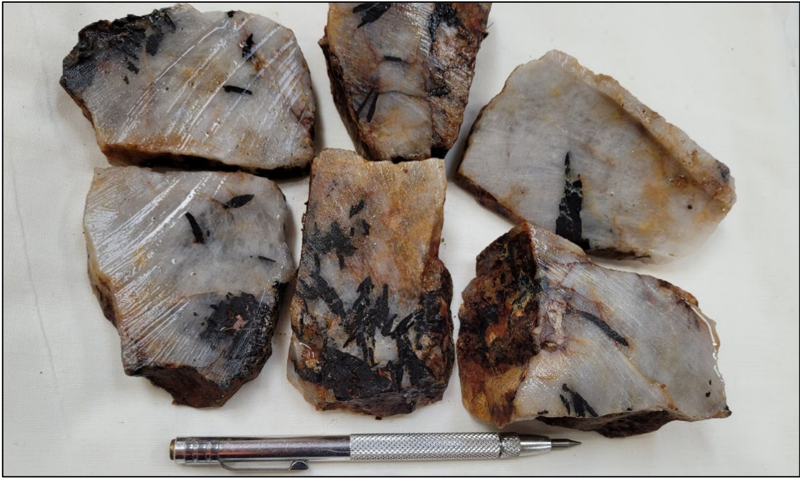
Figure 9 – Rock chip sample 78677 (13.43% WO 3 ) showing visible black crystals of wolframite within a quartz vein.
