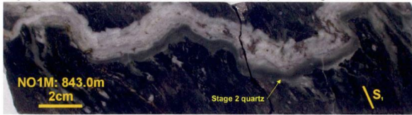
b) Colloform quartz breccia comprising angular sandstone fragments containing Stage 1 quartz veins (centre and top) that have been progressively rimmed by cryptocrystalline quartz-chlorite (in part replaced by stilpnomelane) and crystalline quartz. Cavities and vughs are infilled with pale green partly recrystallised cryptocrystalline quartz.
