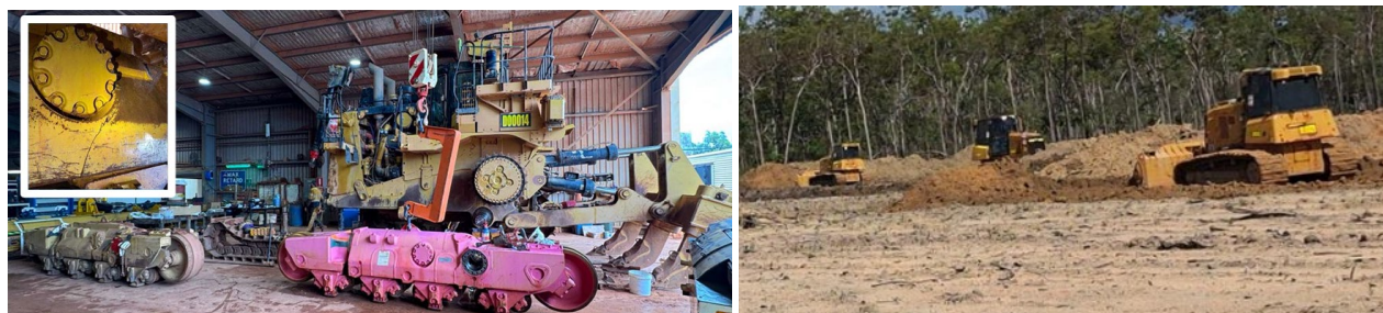
Picture: Replacement of a cracked track on a D10 dozer (L), D4 dozers stripping waste in March (R)
