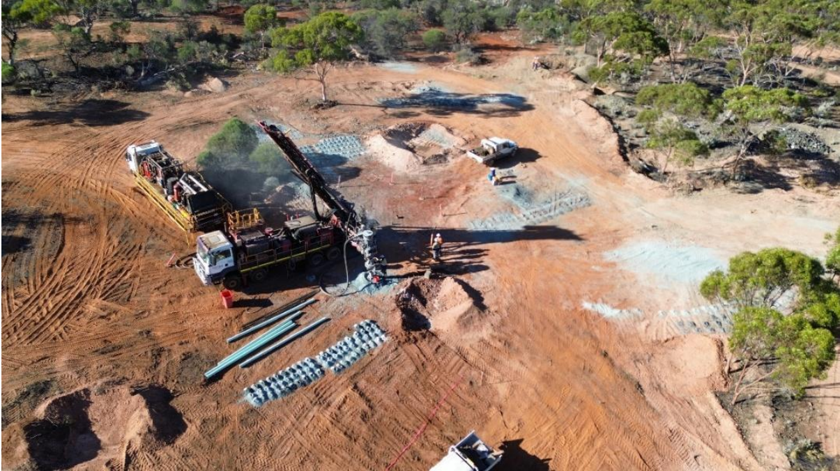
Figure 14: RC rig drilling at Star of Ennuin (historic workings in top right-hand corner).
