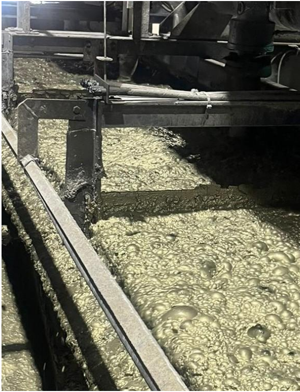
Figure 1 (a) and (b): Copper flotation (bubbles) and the resultant copper concentrate.
