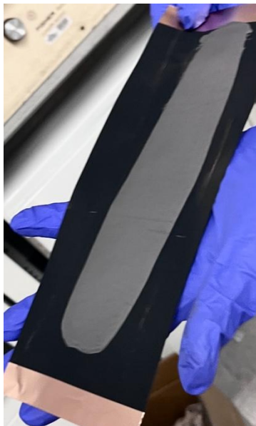
Figure 1 SiNTL™ anode material coated onto copper foil using conventional slurry-based processing methods, demonstrating compatibility with standard lithium-ion battery manufacturing.
