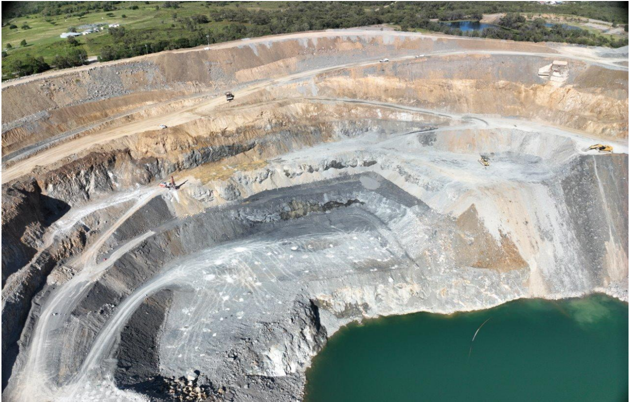
Mining operations advancing on the south wall early April, with next blasts in the 325-315 RL level
