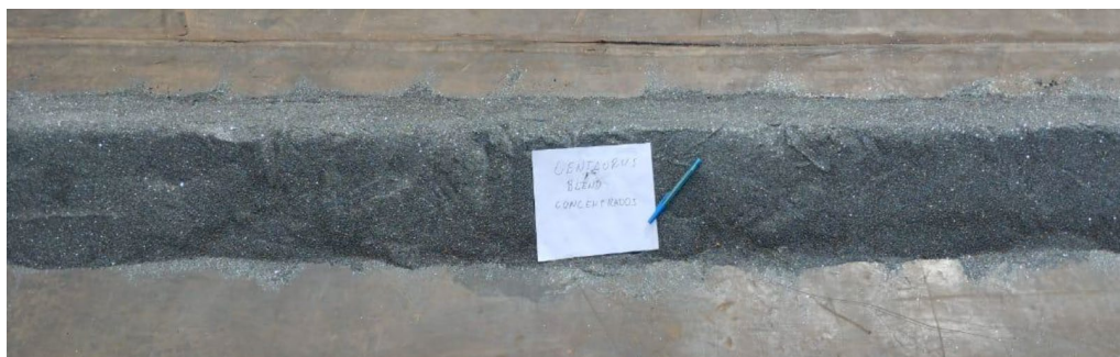
Figure 7 – Jambreiro DR-quality concentrate produced from pilot plant
