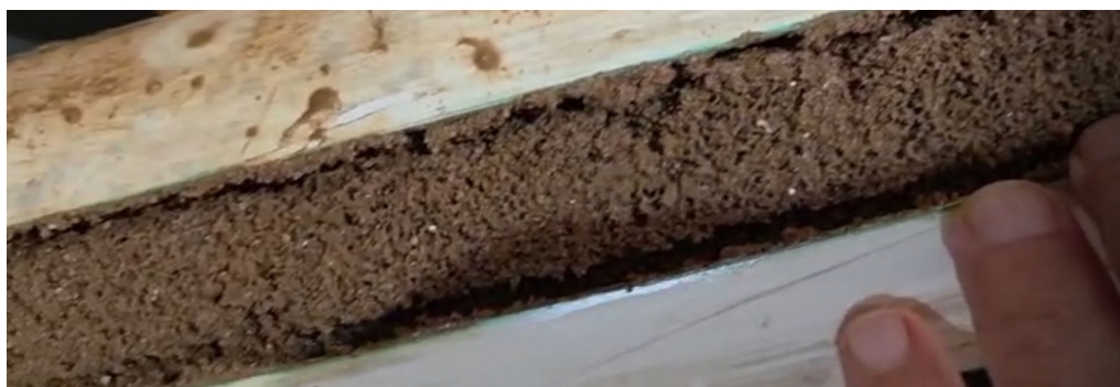
Figure 8 – 90% Rougher spirals tails + 10% thickened slimes after natural free draining test
