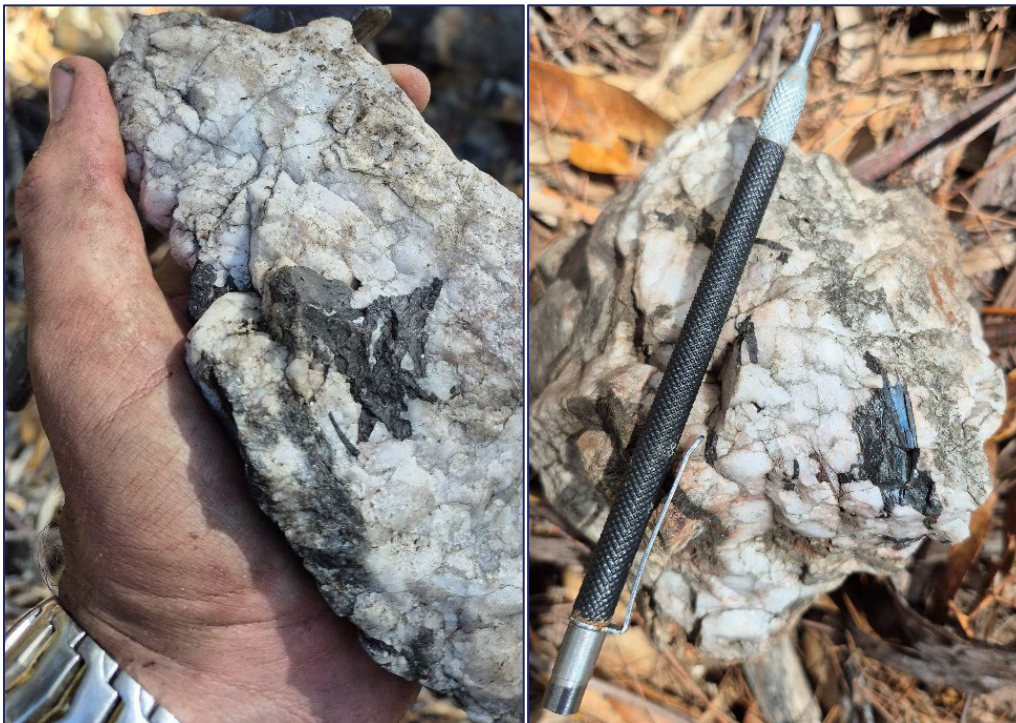
Figure 1: Coarse wolframite crystals hosted by quartz veins at the Lutwyche Prospect, Scamander Project (Samples LW26013 (Left) and LW26006 (Right))
