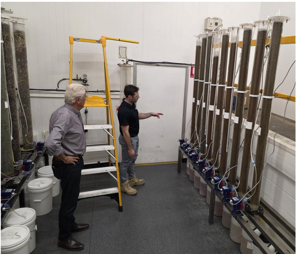
[Figure 1] Sybella Project: Two metre column leach test work in progress.
