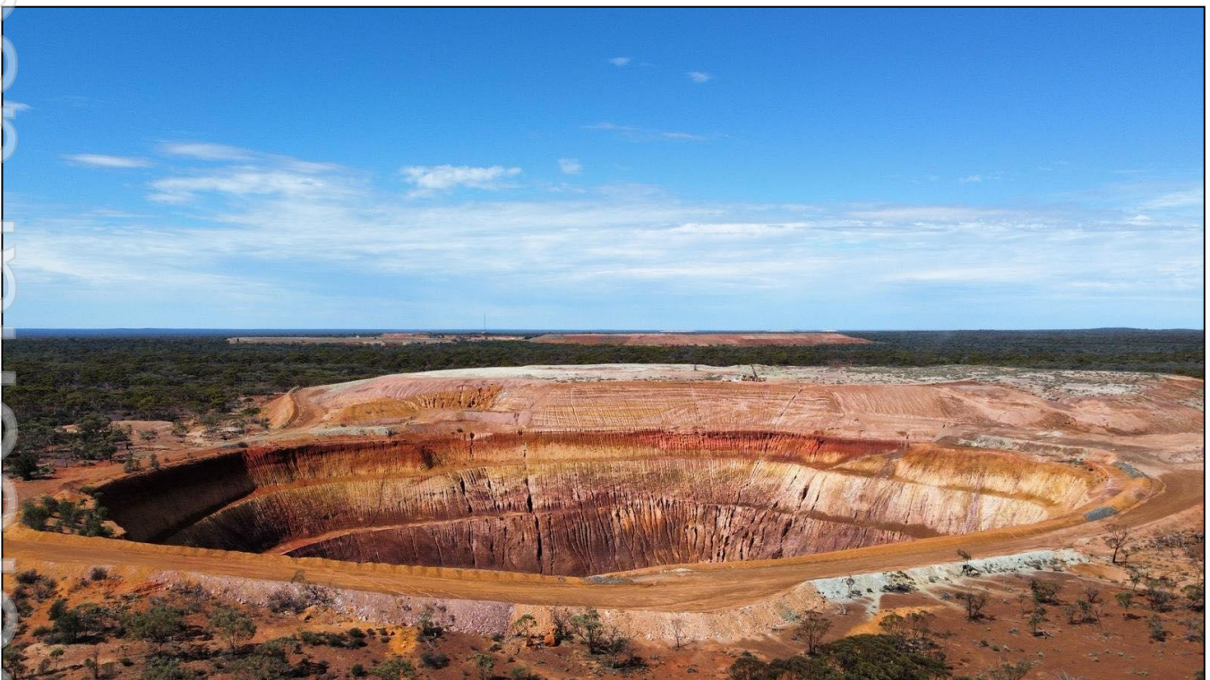
Figure 1 - Eureka open pit, aerial view looking east. Note the excellent wall condition
