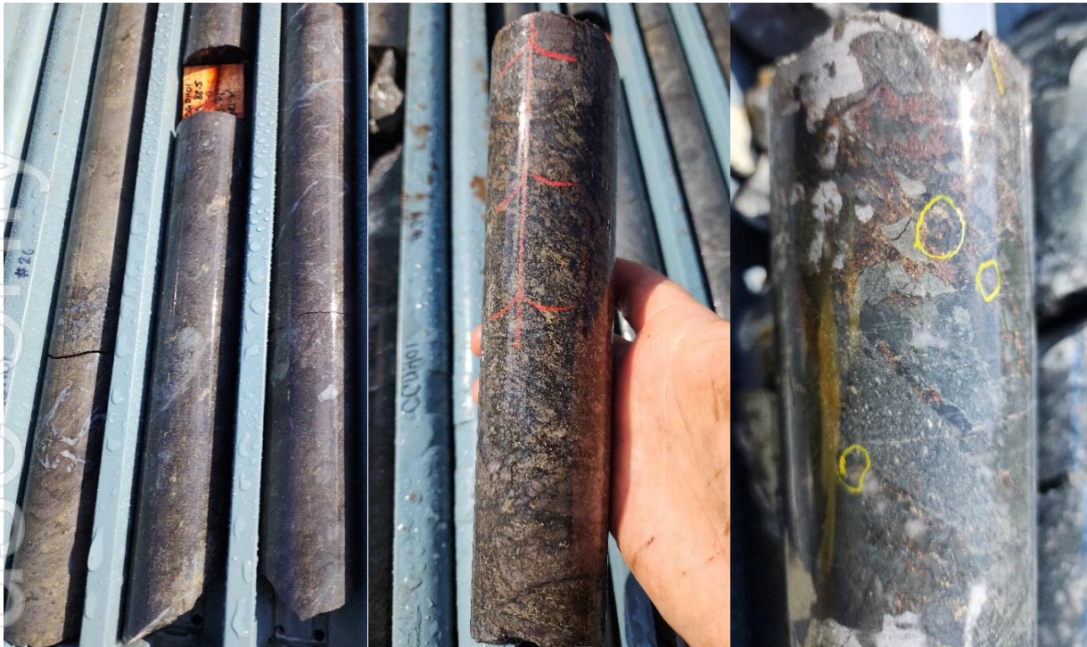
Figure 2: A Sphalerite, chalcopyrite and pyrite with silica and carbonate alteration intersected in CGDH001 in the hanging wall of the Christmas Gift gold orebody 2 .
