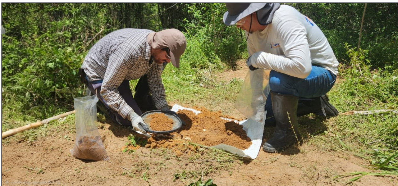
Figure 2: Auger drill sample preparation and sieving at the Itambe Project, Bahia State Brazil.
