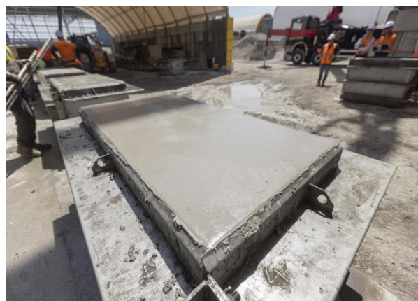
Figure 1 & 2: Wind farm concrete trials - 50% AusPozz™ mix design
