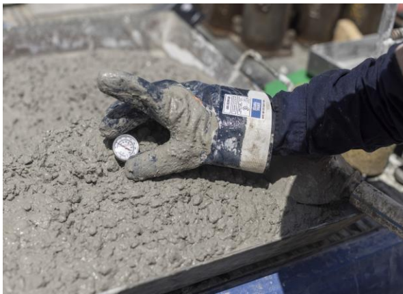
Figure 1 & 2: Wind farm concrete trials - 50% AusPozz™ mix design
