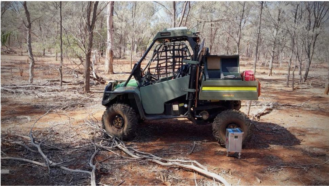
Figure 6. Collecting Gravity data on the Byrock Project (March 2026)
