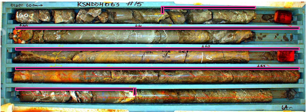
Figure 4: KSNDDH063 core photos with massive sphalerite and galena mineralisation. Interval highlighted in pink; 3m @ 12% Pb, 16% Zn, 195g/t Ag from 60.5m.
