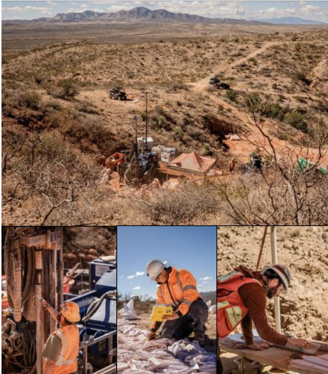
Figure 2: Clockwise from top. Midnight Sun’s Grasshopper RC rig drilling RBRC026. Company geologist inspecting RC chips. Field technician collecting magnetic susceptibility measurements. RC drilling rod change.
