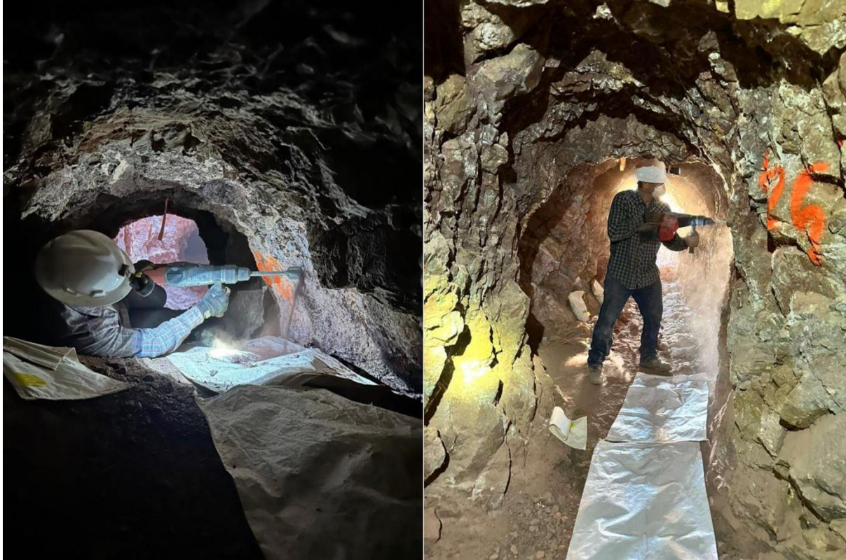
Figure 4: Underground chip-channel sampling with demolition hammer and chisel bit at Red Bird.
