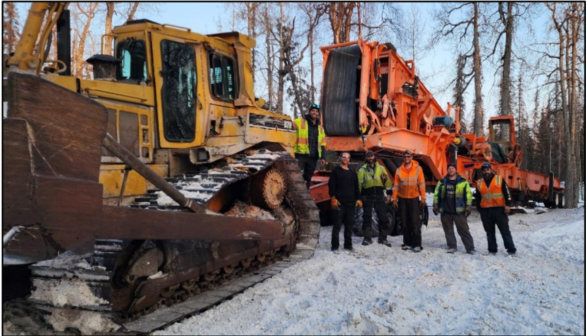
Figure 7. Screener plant being delivered to site via the winter snow road
