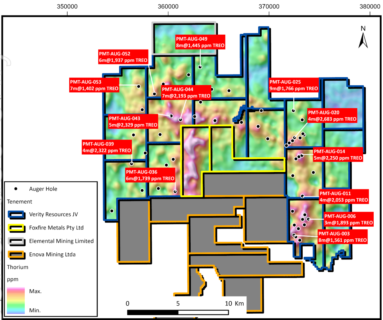
Figure 9. Pimenta Project with significant TREO intercepts, over airborne radiometric image.
