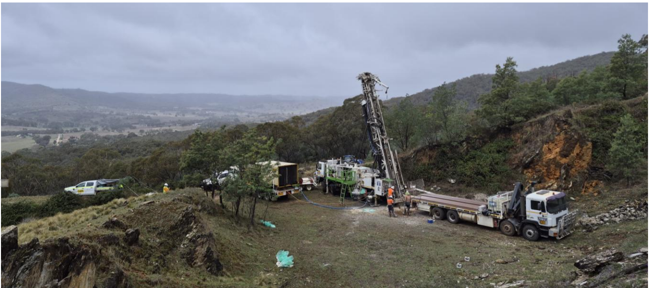
Figure 5: Photo of reverse circulation drill rig on site and drilling at Lewis Ponds
