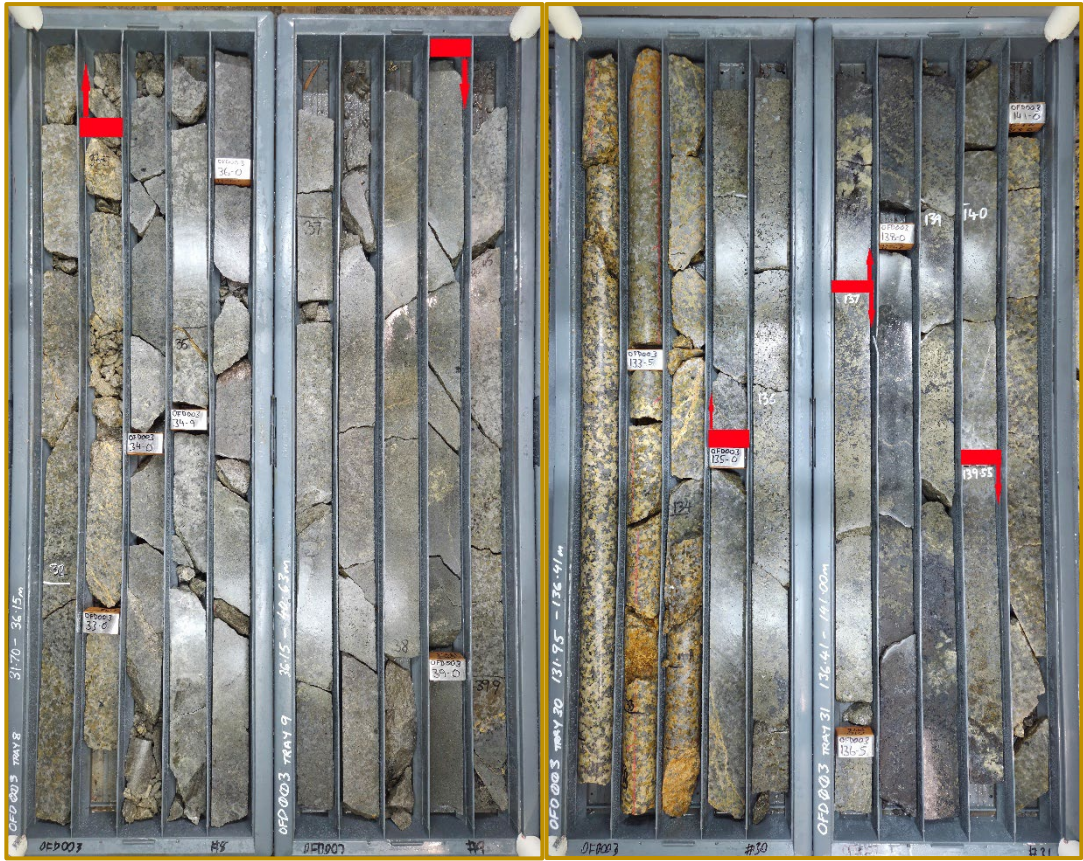
Photo 2 & 3. Sweeneys Drillhole OFD003 Core Tray showing granite host rocks with sulphide lodges observed at depths of 33.55 – 39.80m and 135-139.55m.
