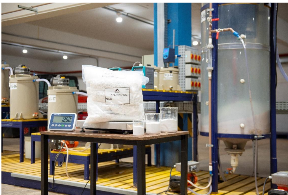
Figure 2: MREC final product and MREC bed (~20cm high) shown in the thickener.
