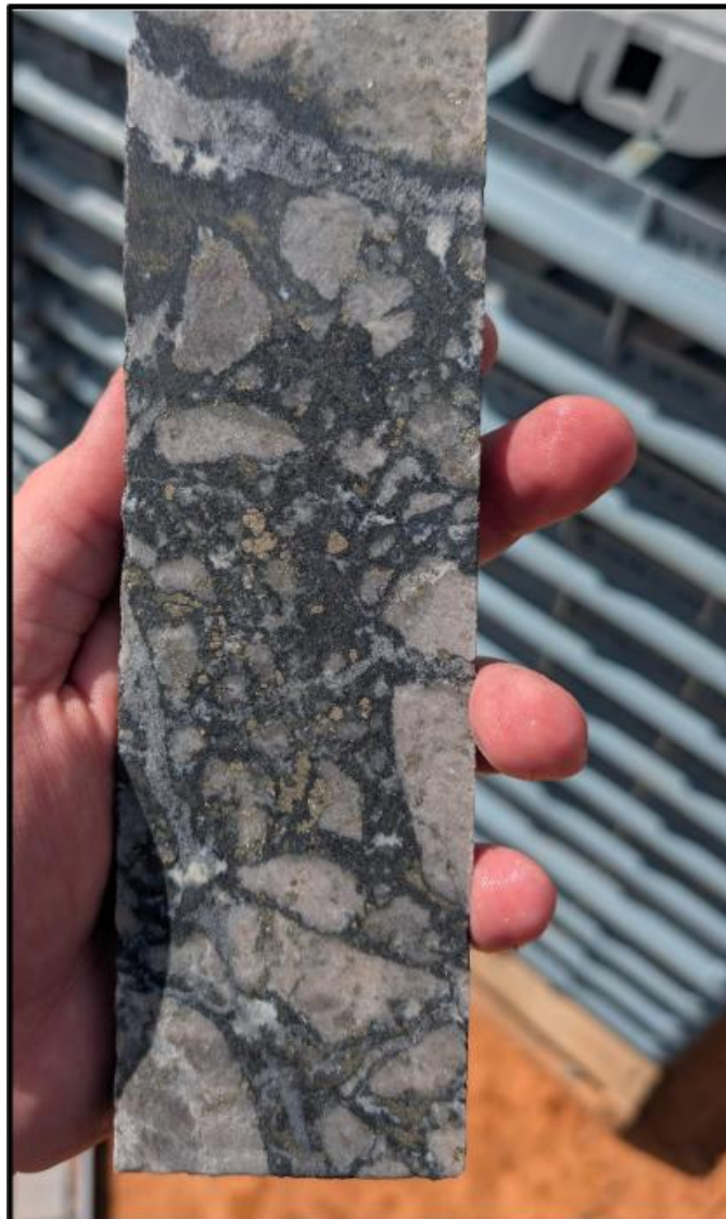
Figure 3: Representative drill core from MMDD007 (171m), mineralised enargite-pyrite hydrothermal breccia within vuggy residual quartz. Pale silica altered clasts are cemented by dark sulphide enargite rich matrix with abundant brassy pyrite. Photo: QMines. 2
