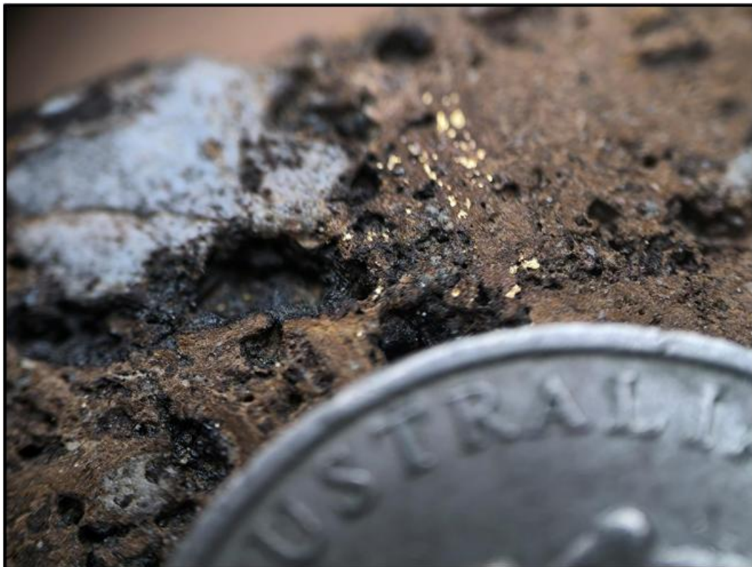
Figure 2: Visible gold in hole MMDD010 at ~11.20m with 10 cent piece, Mount Mackenzie, Vein 355. 1
