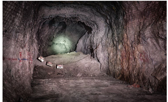
Figure 2: Open stope following blasting
