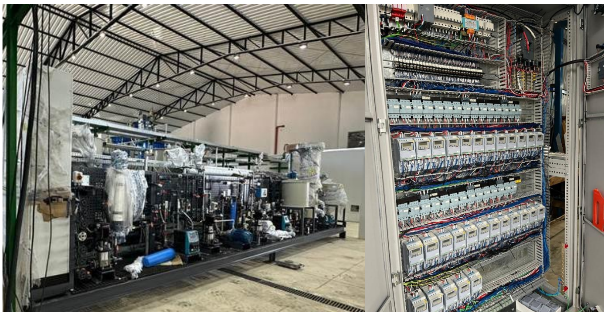
Figure 2: Water treatment and recycling skid delivered and stored at the CPTR on the left and fully integrated Programmable Logic Controller (‘PLC’) control system designed to control and provide data from the demonstration plant on right.
