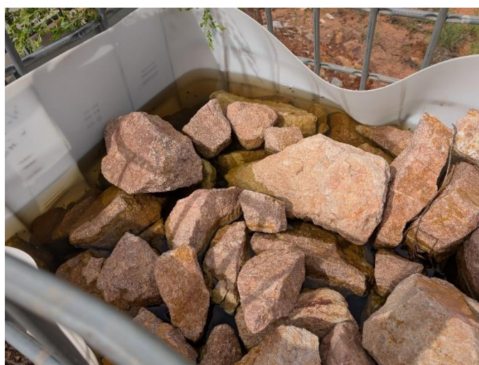
Figure 1: Kinetic leach trial testing for closure planning.
