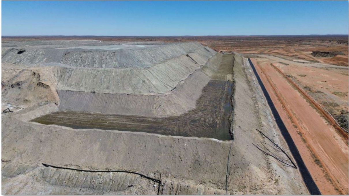
Photo 1: Cyanide irrigation underway along western side of heap leach pad at White Dam Gold Project in South Australia
