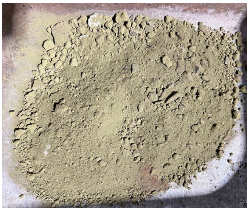
Photo 4: Stripped and calcined gold product (circa 90% Au) from first carbon stripped at White Dam
