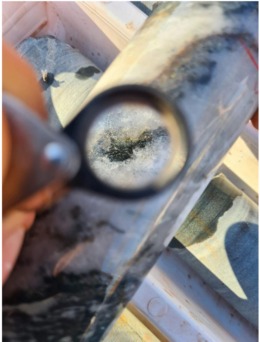
Figure 1: Image of coarse free gold from MZDD001: 76.8-77.0m which assayed 40 g/t Au. Field of view within hand lens ~2.5cm.
