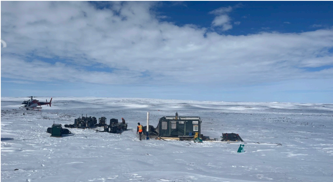
Figure 5 - Photograph of reverse circulation drilling rig on DAN26007, highlighting the flat topography and minimal snow coverage.
