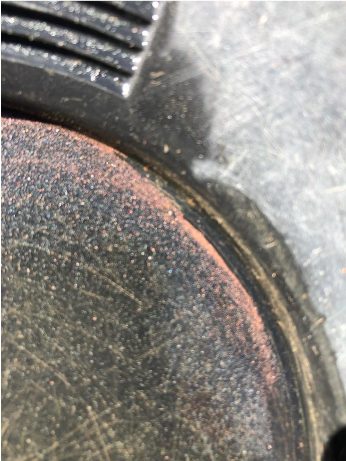
Photo 2. Panned tail showing native copper (pink colour) from drill chips from YRC26-23 (97m to 98m)
