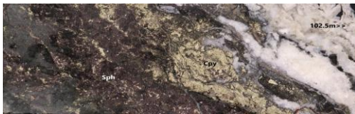
HVD003, 102.3 - 102.5m semi-massive chalcopyrite and sphalerite
