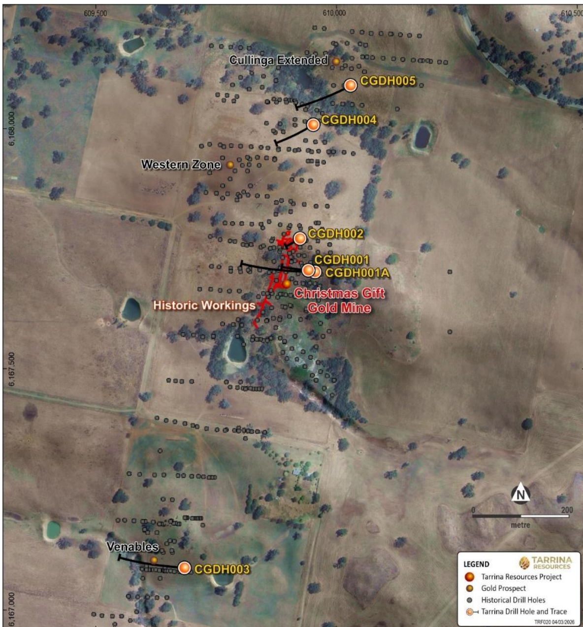
Figure 1: Location of diamond drill holes in relation to historic drilling and Christmas Gift mine workings.
