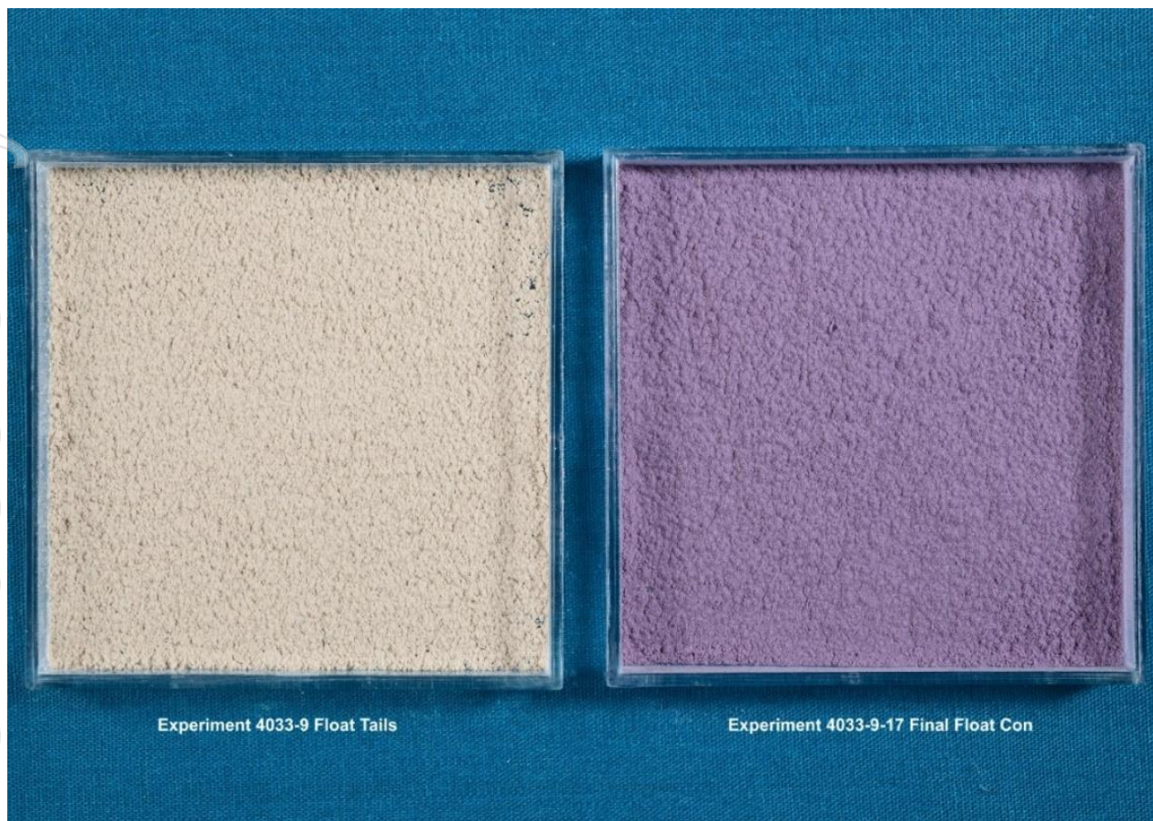
Figure 4 Final Flotation Concentrate and residual tails
