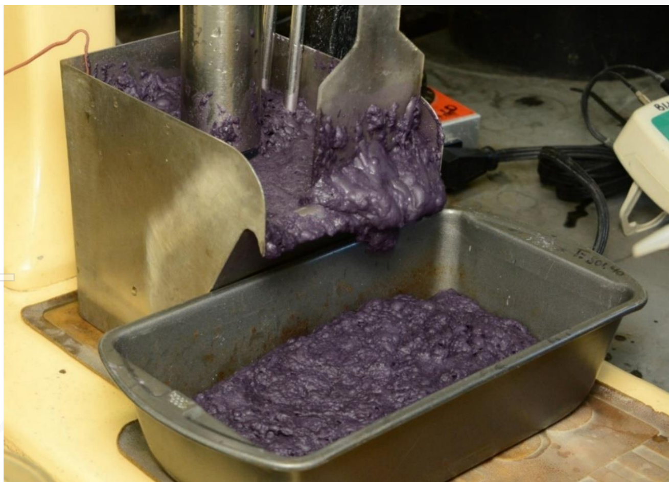
Figure 3 Flotation cell and recovered \text{CaF}_2 froth
