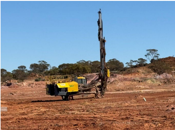
Image 2: Drilling at Redcastle Gold Project including blast holes for mining
