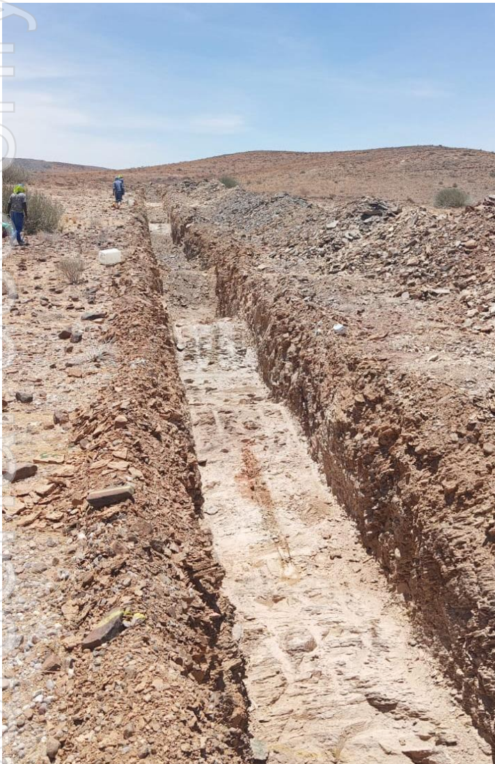
Image 1: Example of the trenching completed at the PS Target. Trenches are dug using a mechanised excavator to the point of refusal. The trenches are then cleaned manually and mapped by a geologist to document the exposed geology across the width of the pegmatite target and document the host lithology. Visual indicator marks are made across the pegmatite for channel sampling to be completed using a rock saw and hand chisel to remove the sample for bagging and sample preparation.
