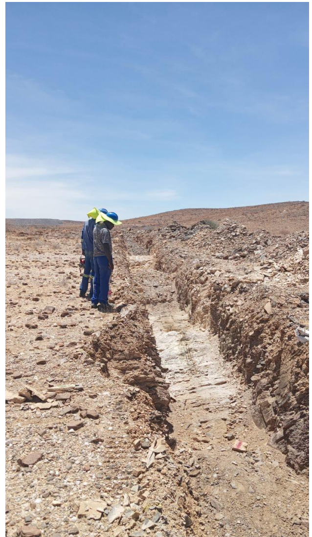
Image 2: Example of the channel sampling completed at the PS Target using a rock saw and hand chisel to remove the sample for bagging and sample preparation.
