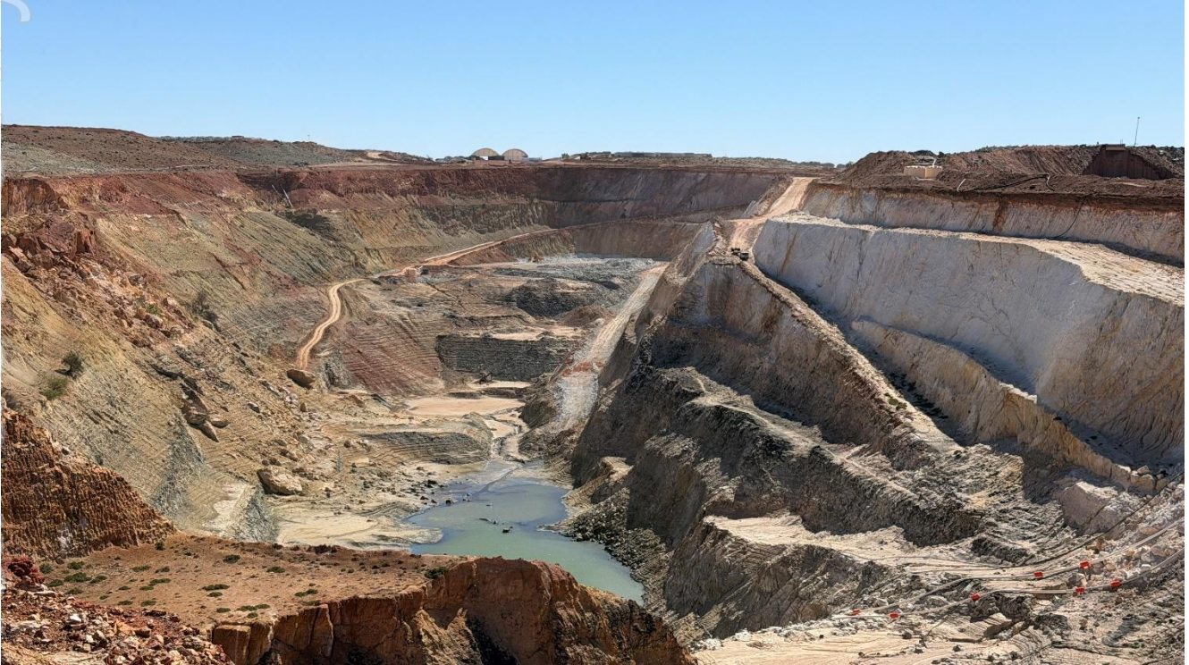
Figure 1 – Youanmi Main pit dewatered (looking North) – now at limit of pit pumping
