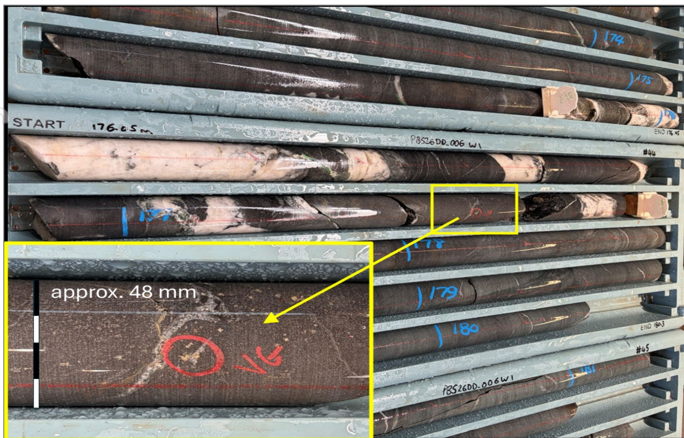
Figure 3: Visible gold ('VG') in PBS26DD_006W1 which assayed 0.5m @ 41.98 g/t Au from 177.2m. This interval is in the footwall (i.e. below) and unrelated to the main 050 Structure at Paringa West (see cross section in Figure 5 ).
